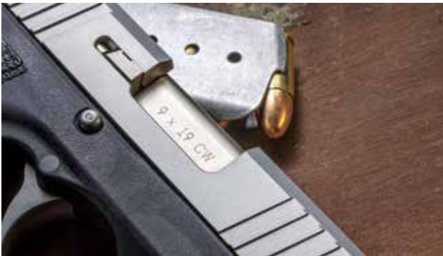
The S9 operates using a John Browning-inspired recoil lug and locked-breech concept.
