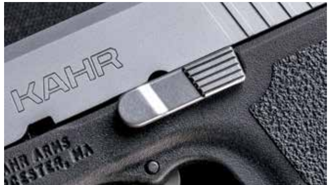
The only lever on the left side is the slide-lock, which is pressed out from the opposite side to remove the slide from the frame.
