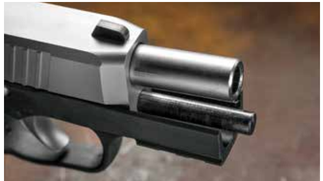
The 3.6-inch stainless barrel tilts up when unlocked and is tight at the muzzle when the slide is forward.
